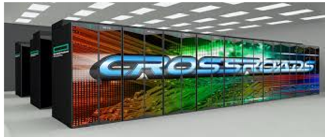
LANL ATS System Crossroads Installed 2023 - power consumption is a maximum of 18 MW, 6,144 compute nodes
