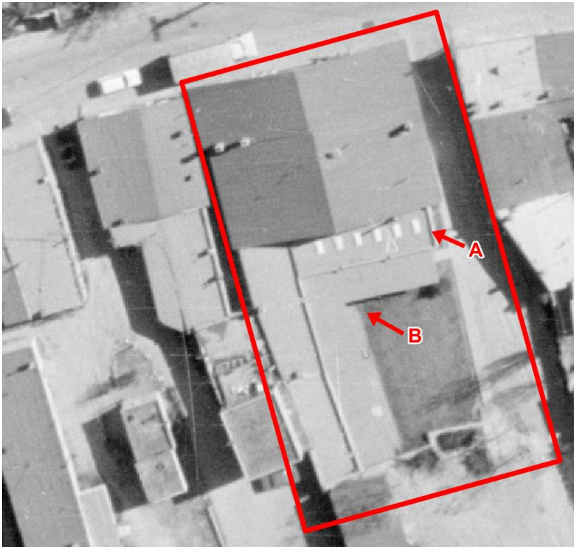
Figure 7: May 11, 1973, aerial photograph. A. ground-level addition; B. structures of wing unified under one roof; portal is present.
