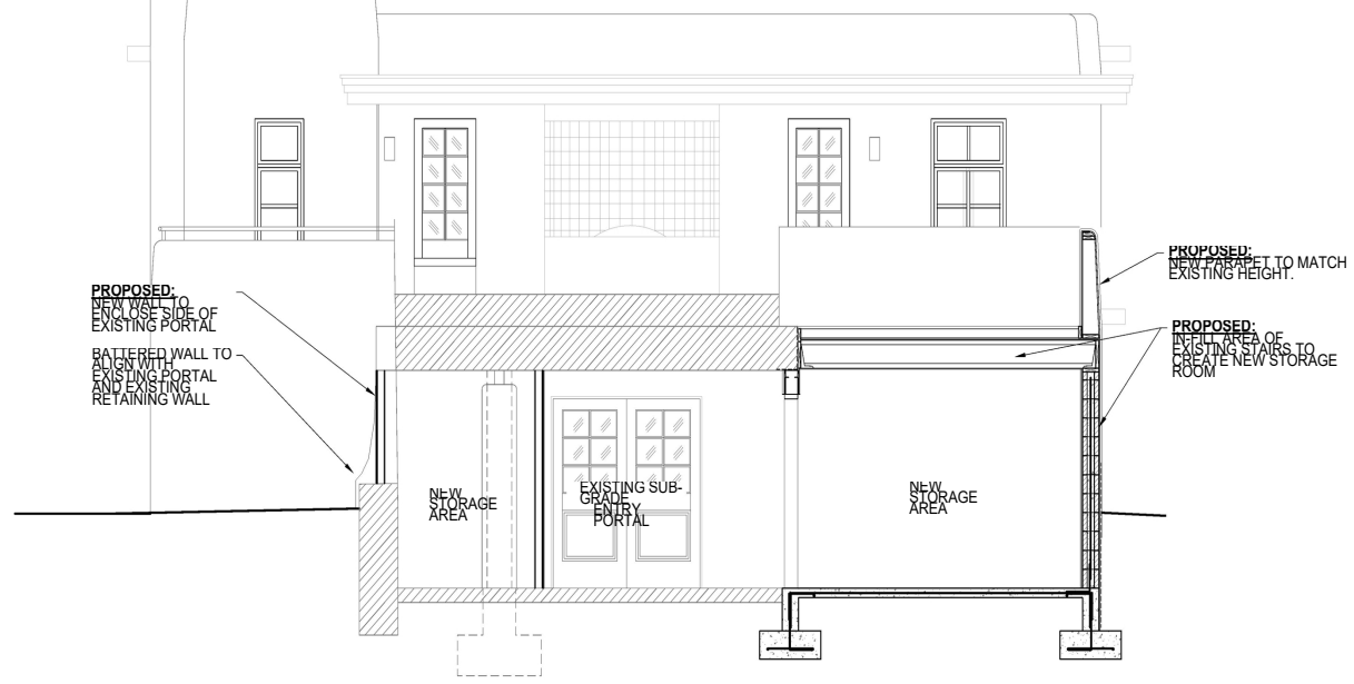
2 PROPOSED SECTION THROUGH NEW STORAGE SPACES
