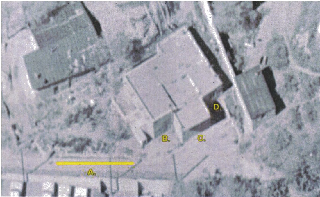
Figure 3: May 11, 1973, aerial photograph. A. wall present, though then longer in length; B. current wood casement window not shown; C. bump-out present; D. window is shown where a door is now. Courtesy NMDOT, State of New Mexico.
