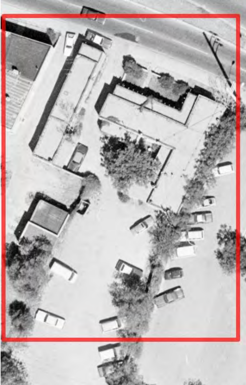
Figure 7: September 11, 1978, aerial photograph. Note likely enclosure of rear entrance at 1121 and removal of frame garage at 1123. Note addition has not been constructed on east side of 1123. Note also cleanup of site and use of back area for parking, signaling conversion to commercial use.
