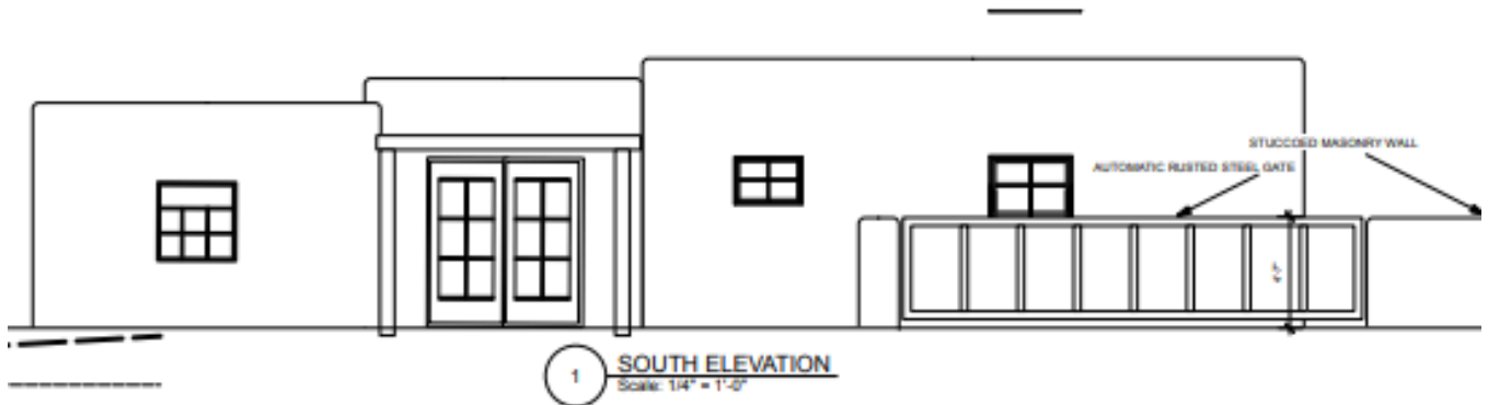
Figure 6. Existing Metal Gate.
