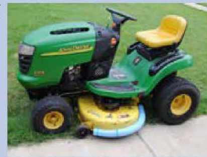
Figure B. A pool ‘noodle’ can be fitted to the deck of a lawnmower to prevent damage to grave markers. Photo: Debbie Dietrich Smith.
