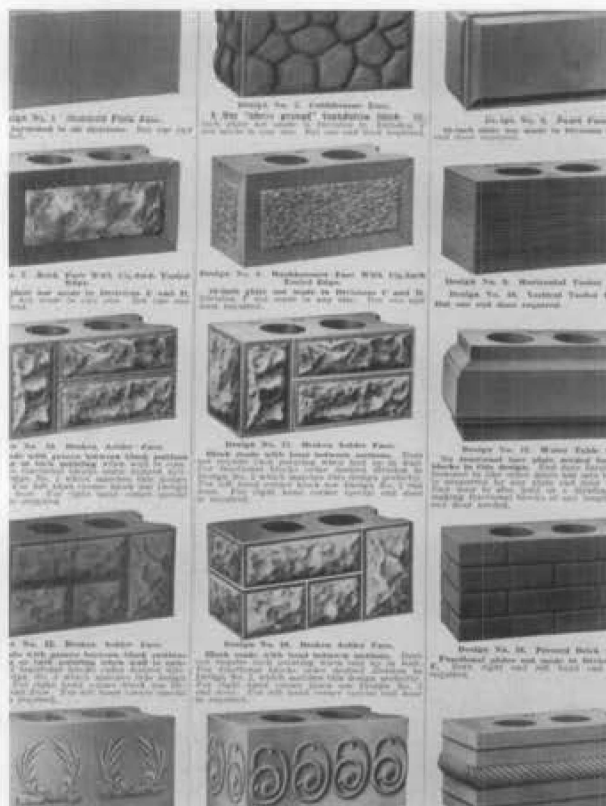
Figure 4. As shown in this Sears, Roebuck and Co. concrete machinery catalog, artistic concrete used standard concrete mixes to produce precast and cast-in-place concrete in molded forms, but made little effort to simulate natural stone.
