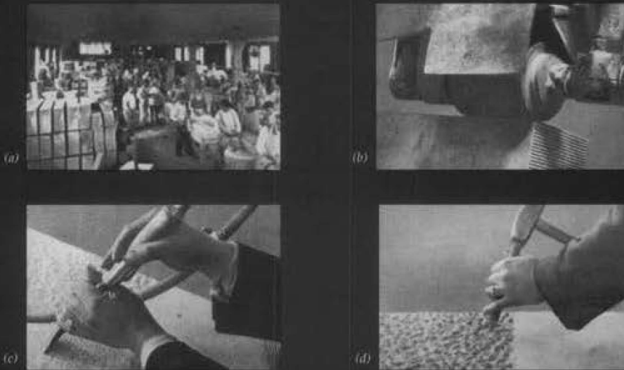
Figure 9. Onondaga Litholite Company Catalog: (a) Section of Hand-Finishing Department. (b) Tooling machines are set up with a series of carborundum wheels that grind grooves into the surface of the stone. (c) Pneumatic hammers are used to produce six or eight cut finish. (d) Point Finish is put on with a single pointed chisel. Courtesy, Collection of Michael F. Lynch.
