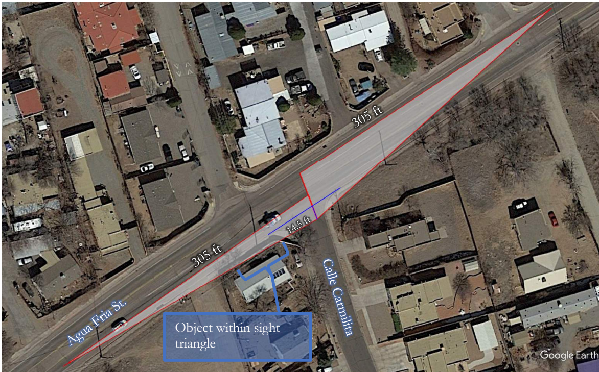
Figure 22: Intersection #7 – Agua Fria Street and Calle Carmilita. Northbound Approach Sight Distance
