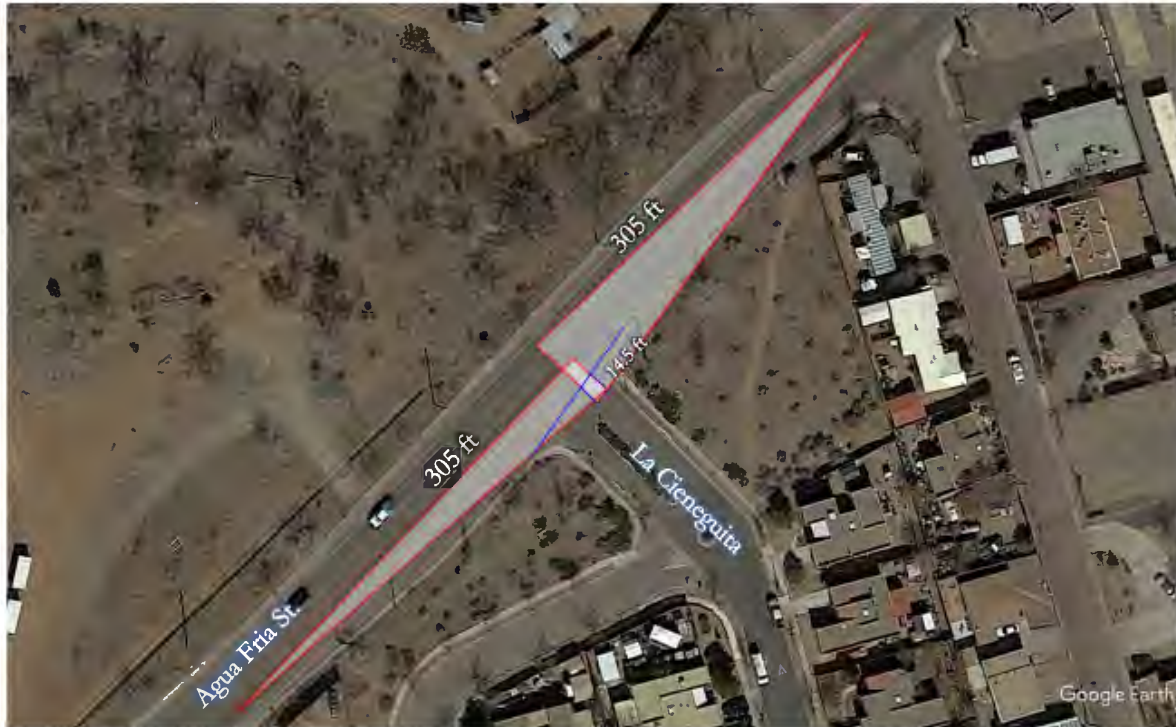
Figure 16: Intersection #4 – Agua Fria Street and La Cieneguita Northbound Approach Sight Distance
