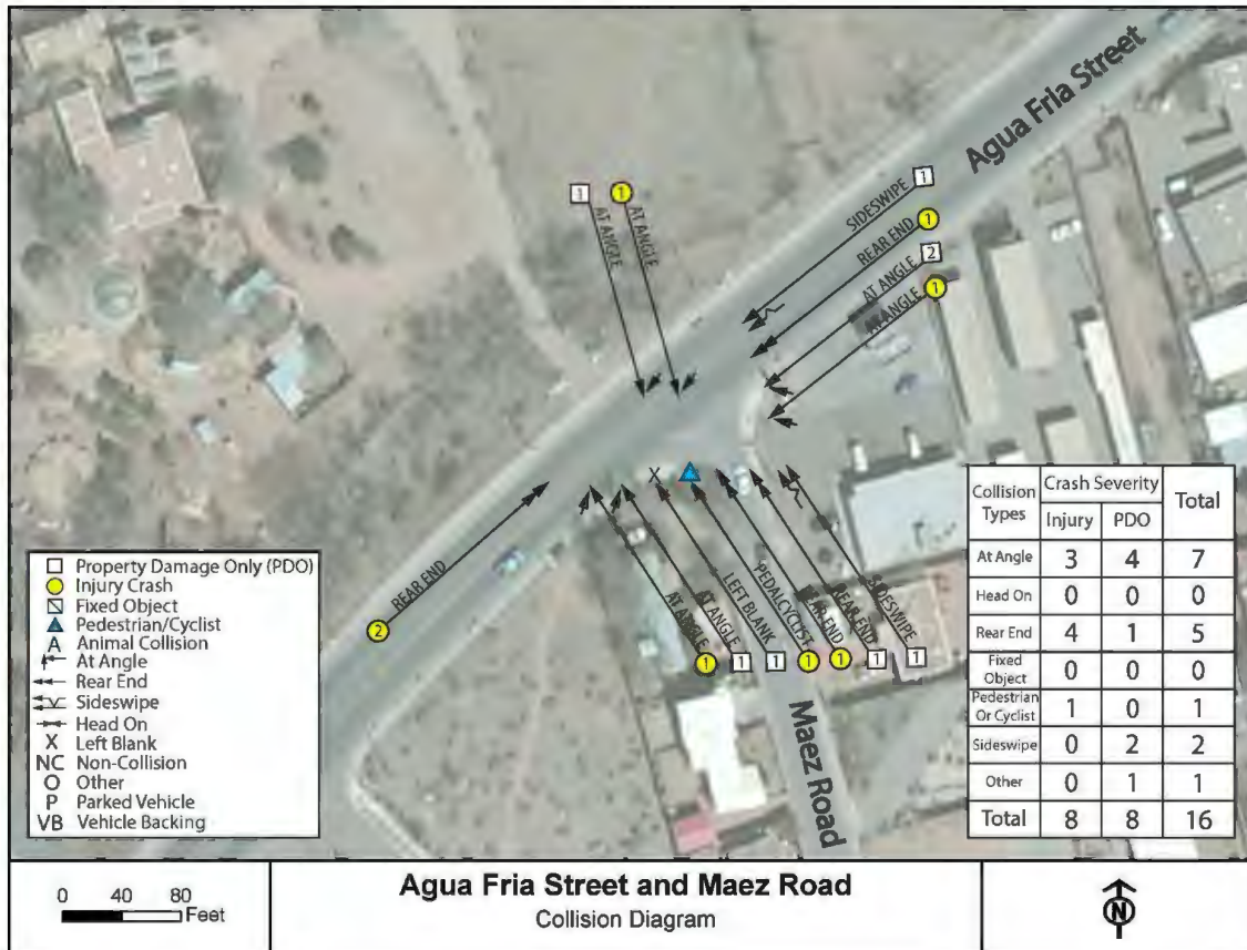
Figure 17: Intersection #5 – Agua Fria Street and Maez Road – Crash Types and Crash Severity
