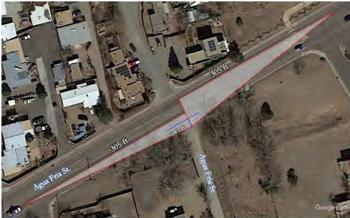
Figure 25: Intersection #8 – Agua Fria Street and Agua Fria Street Northbound Approach Sight Distance
