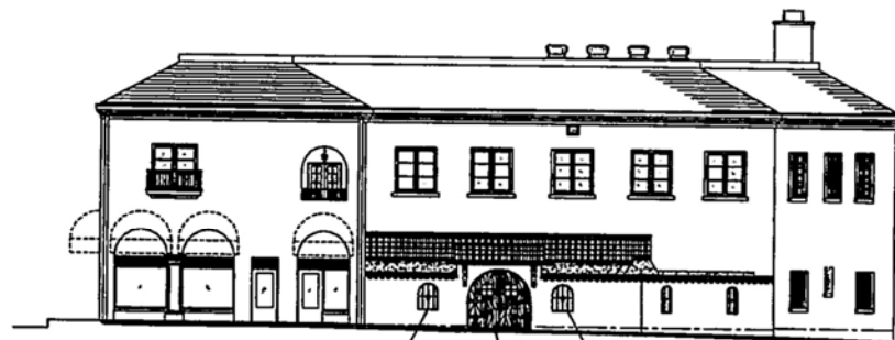
NEW ARCHES NEW GATE NEW ARCHES 4 PROPOSED NORTH ELEVATION - WATER STREET SCALE 1/8" = 1'-0"
