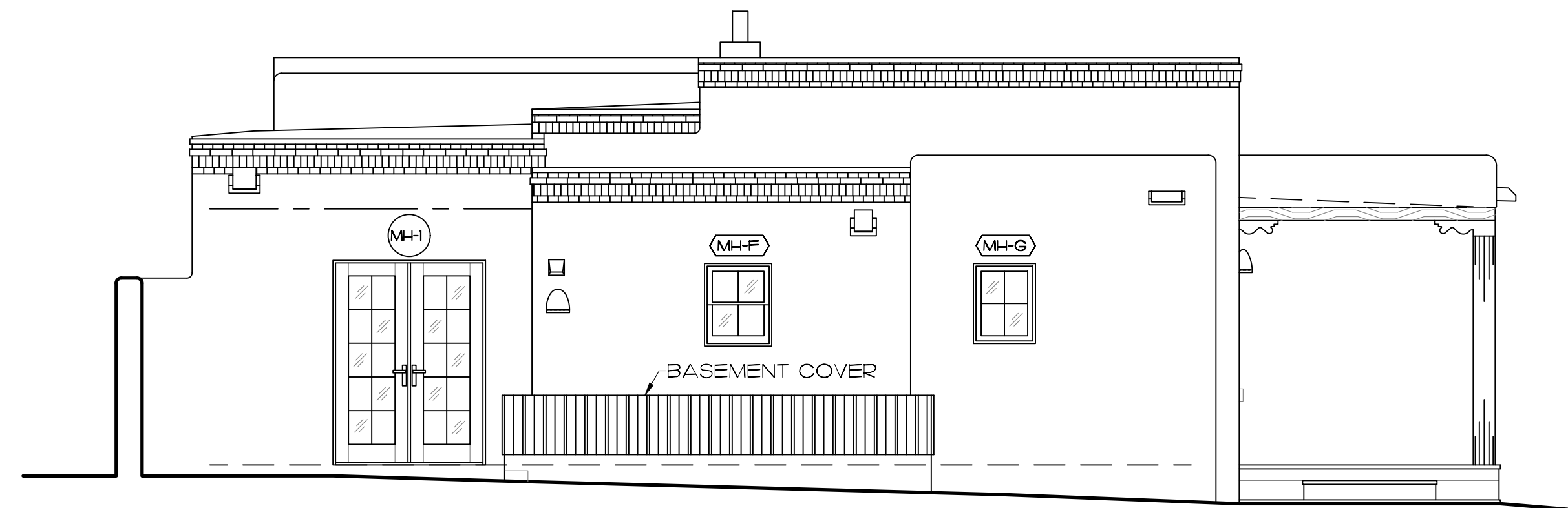
3 EXISTING EAST ELEVATION - MAIN HOUSE A-3.0 SCALE: 1/4" = 1'-0"
