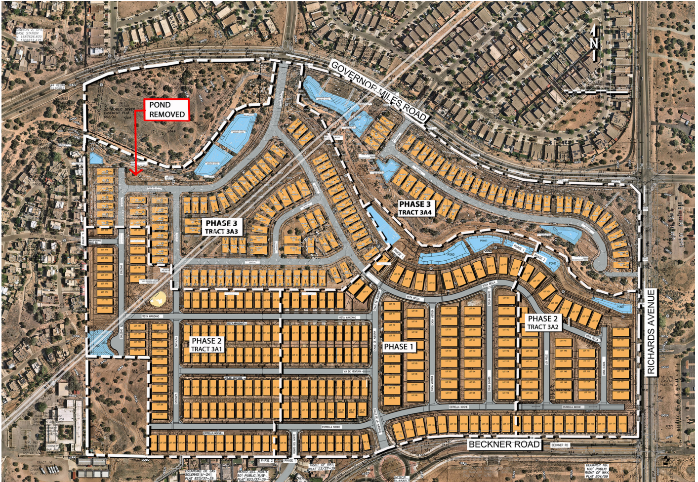
Figure 12- Stormwater Ponding Areas
