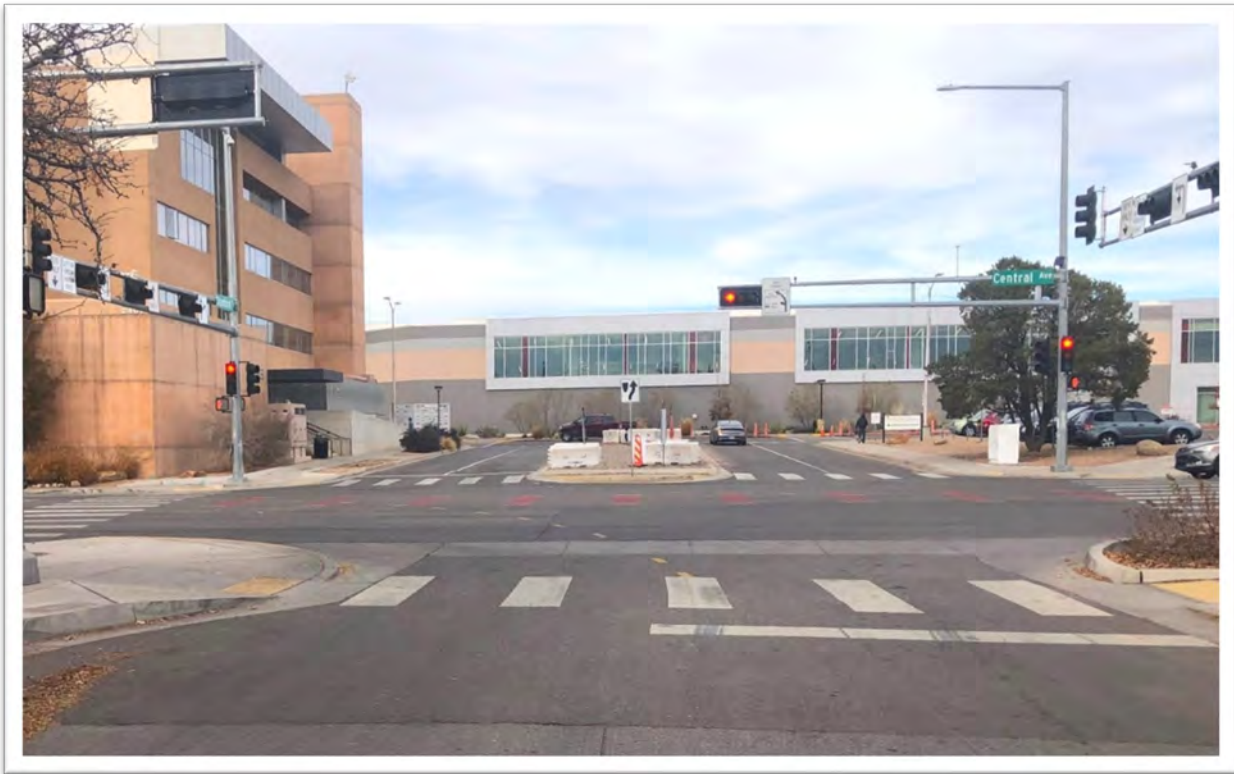
Figure 56: Curb Extension at Signalized Intersection
