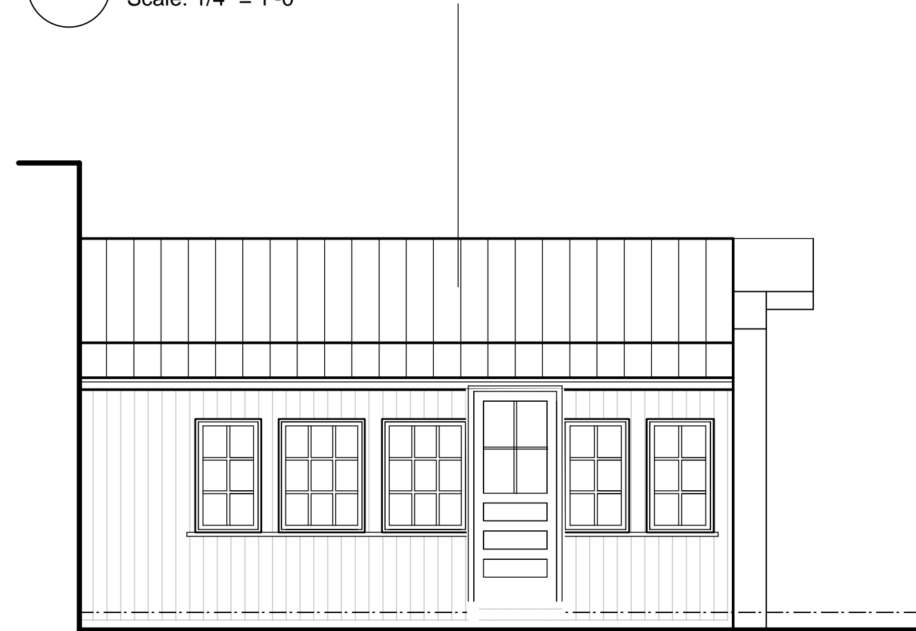
2 NORTH ELEVATION EXISTING Scale: 1/4" = 1'-0"
