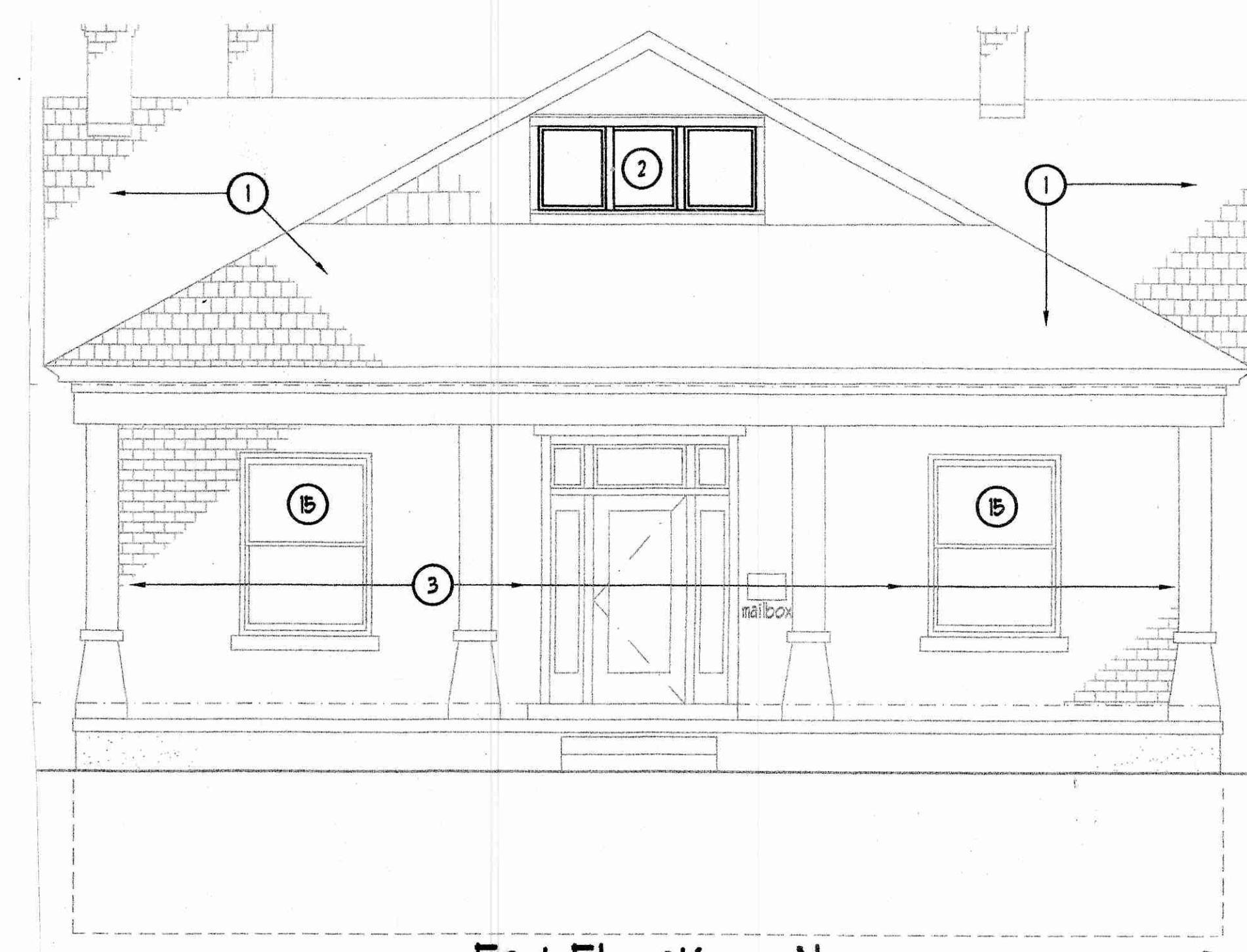
East Elevation - New 1/4"=1'-0" 2 A3
