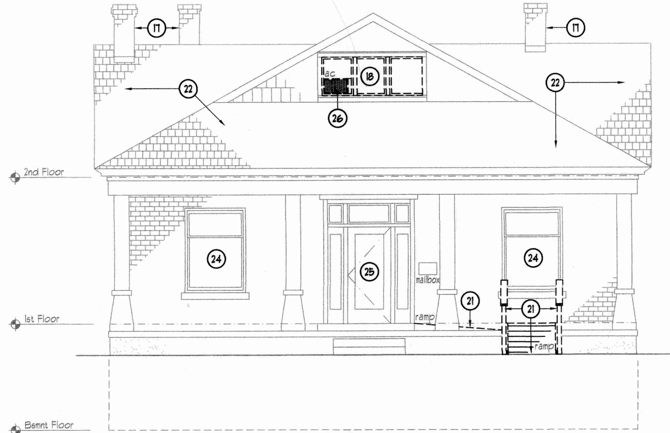
East Elevation - Demolition 1/4"=1'-0" 1 A3
