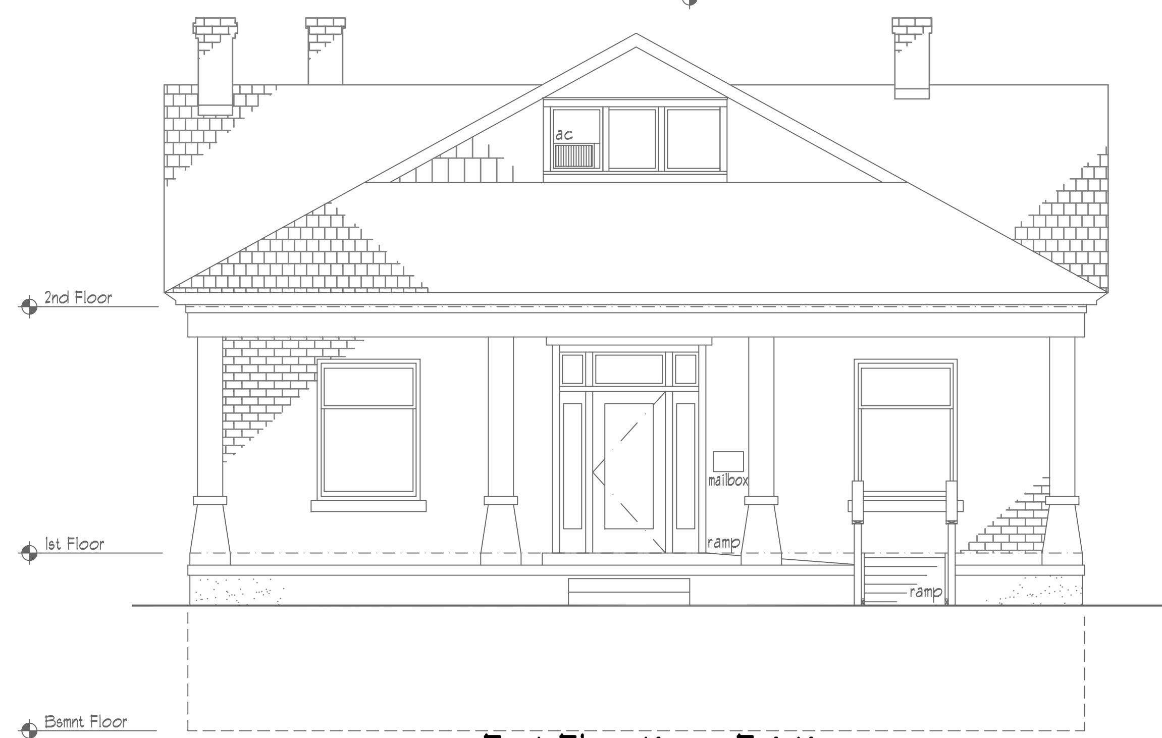
East Elevation - Existing 3 1/4"=1'-0" A4
