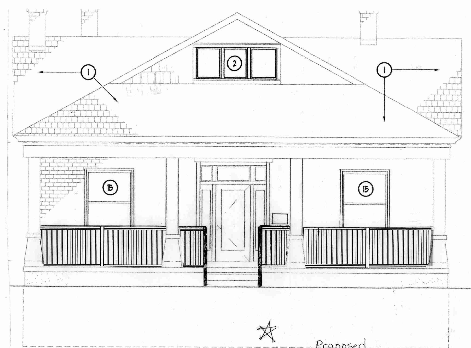
East Elevation - New Safety Rail 1/4"=1'-0" 3 A3 Proposed City Required to match Back Porch
