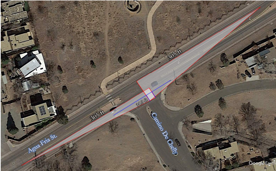
Figure 27: Intersection #9 – Agua Fria Street and Camino De Chelly Northbound Approach Sight Distance
