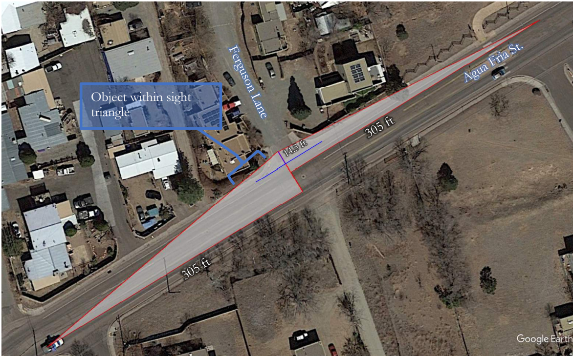
Figure 24: Intersection #8 – Agua Fria Street and Ferguson Lane Southbound Approach Sight Distance
