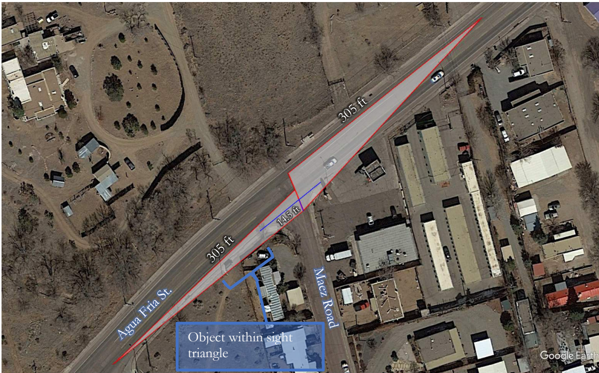
Figure 18: Intersection #5 – Agua Fria Street and Maez Road Northbound Approach Sight Distance
