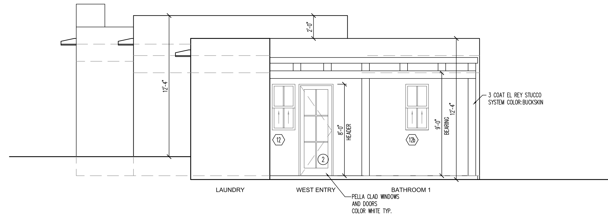
3 WEST ELEVATION Scale: 1/4"=1'0"
