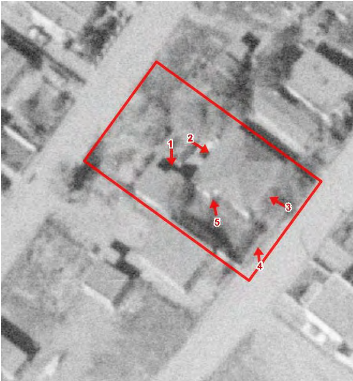
Figure 6: November 10, 1958, aerial photograph. 1). Gabled shed and flat-roof carport; 2) depth of original rear porch; 3) absence of front porch; 4) presence of street wall; 5) presence of bump-out.
