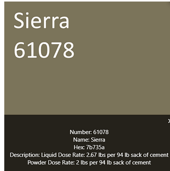
CONCRETE PATIO: DAVIS COLOR SIERRA
